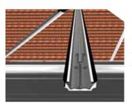
Fully tighten nut on the jack rafter to the eaves beam.
