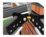
Connect the glazing bars to the D ring and fix down onto the eaves beam. Insert glazing panels around D ring and fit glazing bar top caps.
