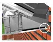
Firstly clip into place the eaves trim to the underside of the box gutter nearest to wall.
