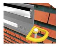
Screw the M10 stud into the half D ring from the under side to allow fitment of the internal half D cover at a later stage. (for clarity the glazing bars are omitted)
