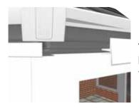
The eaves trim must be fitted prior to the guttering.
