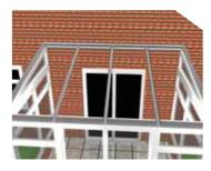
Fit the remaining glazing bars to the wall plate and eaves beam - the bars are numbered as per the layout plan.
