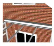
Apply a continuous bead of Silicone between the wall and the wall plate external half ridge cover and the end bar.
