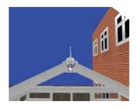
The gable end wall end bars are finished with a cloaking trim and a gable end plate.
