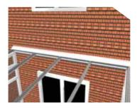
At this point the lead flashing should be completed on the wall plate and if required on the wall end bars.
