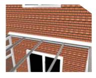
Fix the wall plate external half ridge cover.
