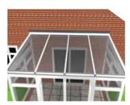
Fit the glazing bar top caps, as numbered on the roof plan.
