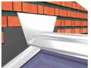
Apply a bead of silicone between the ridge cover and the ridge flashing trim. Slide the ridge flashing trim into the ridge cover. Locate the ridge cover onto the ridge by tapping down with a rubber mallet.
