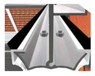
When fitting the glazing bars onto the eaves beam that are connected to the box gutter, it is recommended that the end caps are fitted to the bars prior to fixing to the eaves beam.
