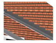
Fit lead into the slots and flashing channel in the wall end bars.
