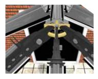
Align the hip bars and any spider bars to the centre line of the D ring (M10 threaded hole denotes the centre line).
