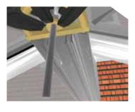
Screw the M10 stud into the D ring from the under side to allow fitment of the internal D cover at a later stage.
