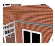
Fix the wall plate to the wall at 500mm centres with propriety fixings at the height shown on the roof plan.
