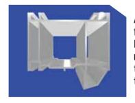
After ensuring the frames are square and level run a line of low modulus silicone along the external rebate in the frame.
