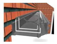
Apply two lines of box gutter sealant on all three surfaces of the box gutter and then slide the connector fully into place.
