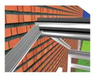
Fix the wall end bars to the eaves beam and ridge, ensuring the ridge is plumb.
