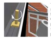
The jack rafter pivot bar should be loosened to facilitate movement, but do not fully unscrew.
