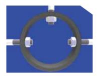
When all of the tie bar stud covers are located pass the tie bar studs into the holes of the aluminium tie bar ring. Secure using the M10 nuts provided.
