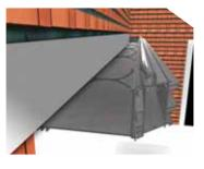
Fit the lead flashing into the slot of the brickwork and fold into the box gutter.
