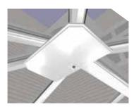
Fit the ridge bottom cladding and internal radius end cover. The internal boss end cover fits to the bottom of the M10 threaded stud situated in the D ring. The nut holding the internal boss end cover should be concealed using the nut cover supplied.
