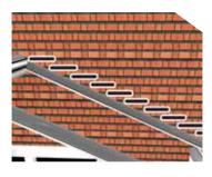
Cut slots into the brickwork to receive the lead flashing above the wall end bars.
