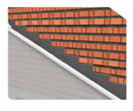
Fit the lead flashing into the cut out slots of the brickwork and fold into the flashing channel of the wall end bar.
