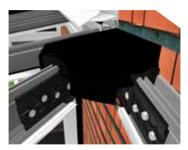
Insert the foam weather seal over the half D ring junction.
