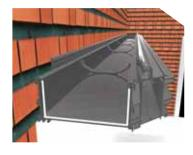
Apply sealant at the joint between the box gutter and the connector. Allow for sealant to set prior to attaching the remaining gutter.
