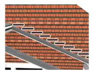
Cut a slot into the brickwork above the wall plate and end bars to receive the lead flashing.
