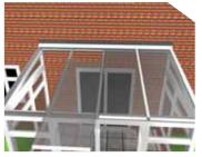
Glaze the panels starting with the panels adjacent to the wall end bars. Ensure the panels are fully inserted into the wall plate and onto the weather strip double sided tape.
