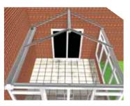
Remove protective film from the bottom caps. Fit sufficient glazing bars to support the ridge.
