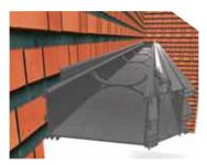
Fix the wall bracket at maximum 600mm centres with propriety fixings. The box gutter and eaves beam can then be hooked onto the wall bracket and secured above the lip of the box gutter with self tapping screws.
