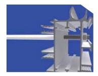
The eaves beam should be pre-drilled from the internal face through to the external face. Insert the horizontal rod through the eaves beam and secure it at the external face with a M10 nut.
