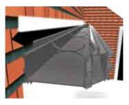
Cut a slot in the brickwork above the box gutter to receive the lead flashing. Apply a bead of silicone along the upper edge of the wall bracket and the host wall.
