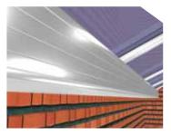
Slide the box gutter under cladding between the eaves trim and the box gutter.
