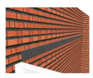
The box gutter wall bracket should be positioned at the host wall with the lower edge sitting 2mm below the window frame height. Ensure the wall bracket is sufficiently packed off the wall to maintain straightness.
