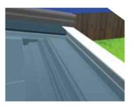
When the glass panel has been positioned the glazing retainer can be rotated upwards until the glass panel is resting on the inside edge of the glazing retainer. Apply a bead of silicone on the top inside edge of the glazing trim and push into the glazing retainer.
