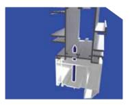
Fix eaves beam to the frames from the inside of the windows using 5.0mm diameter screws at 150mm from the corners and a maximum of 500mm from the centres.
