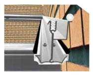
Run a continuous bead of silicone between the wall and the wall end bars.
