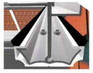
Loosely fit the remaining glazing bars to the ridge and eaves beam, the bars are numbered as per the layout plan, ensure glazing bar centres are maintained on both ridge and eaves beam.
