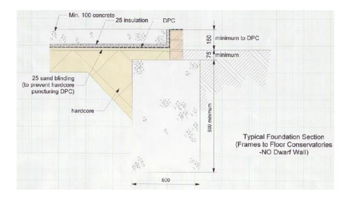
Typical Foundation Section for Full Height Conservatories. (Frames to floor conservatories with NO dwarf wall)
