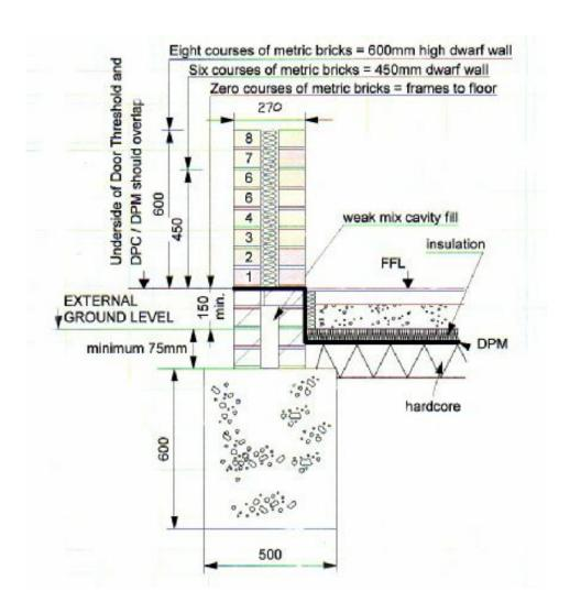
Typical Foundations and brickwork section for dwarf wall conservatories.
