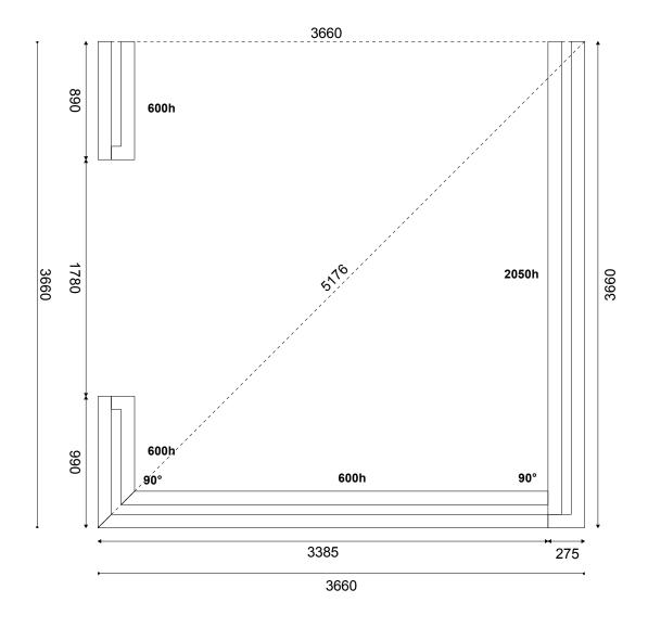
External brickwork dimensions shown. Dwarf wall to be built as 275mm wide cavity brickwork to a height of 600mm from DPC.
